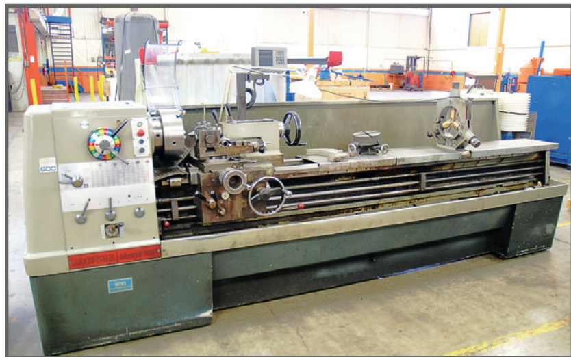
COLCHERSTER MASCOT LATHE, 16" X 110", 12" 3-JAW CHUCK
